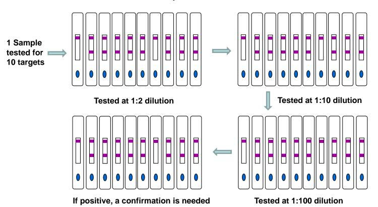
Up to 40 tickets and 4 mL of sample are needed to test a single sample on site!
