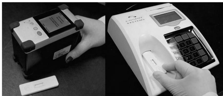
Fig. 2. The NIDS® handheld (left) and medical (right) readers for the quantitative measurement of rapid IM assays.
