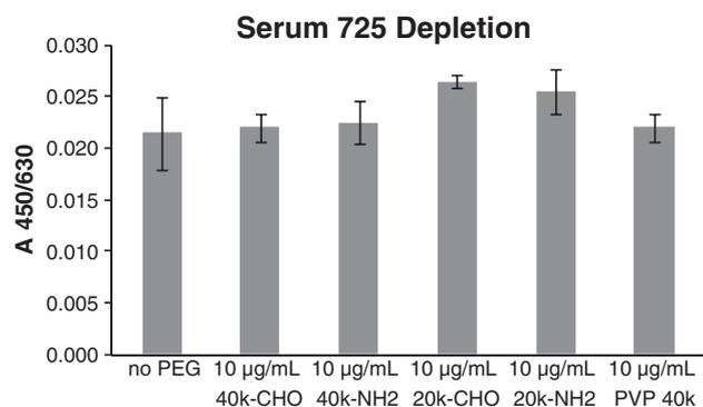
**Fig. 15.** Depletion of sample 725 with 40 and 20 kDa PEG compounds with aldehyde (CHO) and amine (NH<sub>2</sub>) functions and 40 kDa PVP. This sample was a borderline positive which proved to be a true negative.
