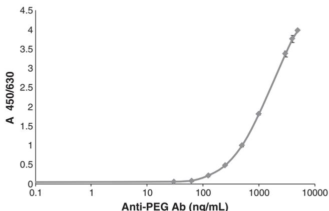
**Fig. 2.** Dose-response curve of the immunogenicity ELISA for the detection of ADA to PEG. The observed limit of detection was 125 ng/mL.
