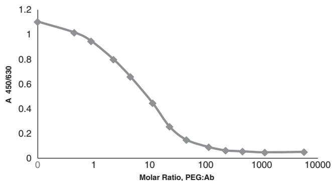
**Fig. 4.** Drug Tolerance of the immunogenicity ELISA using 500 ng/mL of the ANPEG-1 anti-PEG mouse monoclonal IgM antibody spiked into a negative human serum pool. A positive result can be detected beyond 100X excess free PEG. Complete inhibition occurs at a PEG:Ab ratio of 1000:1.
